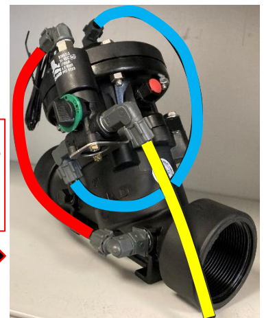
Connecting the tubing to the kit valves (SVO on the left, SV1 on the right). The yellow tube represents the drain in both cases.
