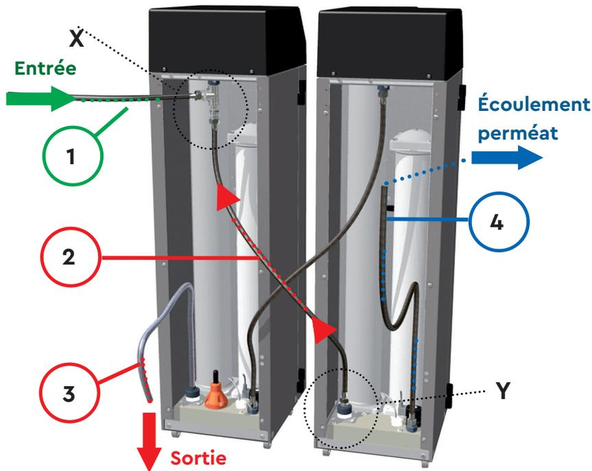
Fig. 16: raccordement hydraulique BWT PERMAQ® Pico Duo
