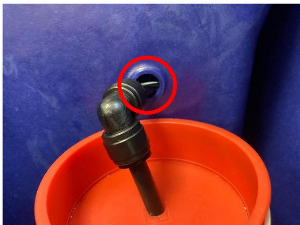
● Pull the pipe to the other side of the tank and connect it to the valve (Item 4 page 34) by making a loop as shown in the photo below:
